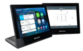
Single integrated controller can operate both ClearOne's audio and video platforms
